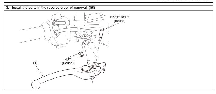
4. Check the lever for proper operation.
